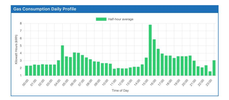
SmartHTC is a measurement of whole building heat loss (also known as a Heat Transfer Coefficient or HTC). It accounts for heat escaping through walls, floors, ceilings and windows as well as infiltration and ventilation losses. The HTC describes the rate of heat transfer from a building per degree of temperature difference between inside and out.
